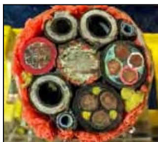
Three inch in diameter, 42-meter unitized umbilical attached from life support buoy to Aquarius. Photo Courtesy of History of Diving Museum, Islamorada, Florida.
