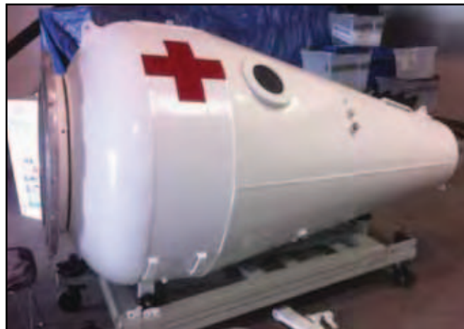
Figure 14. A paramedic and patient containing transport chamber, which is also capable of 6 ATA pressurization and able to fit in the patient compartment of a conventional, land-based EMS ambulance.
