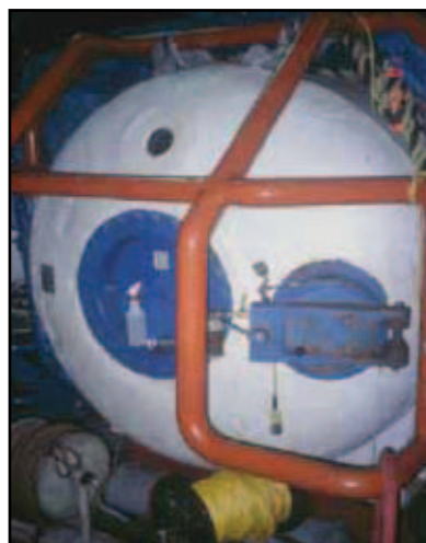
Figure 7. Saturation chamber/diver storage chamber on deck of a commercial diving support ship in which the exsanguinated patient in Case 2 presentation was resuscitated with hyperbaric oxygen therapy.
